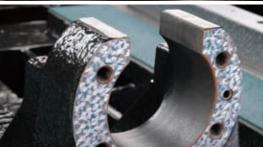
Hand scraped contact areas, minimal axis protection with maximum stroke.
