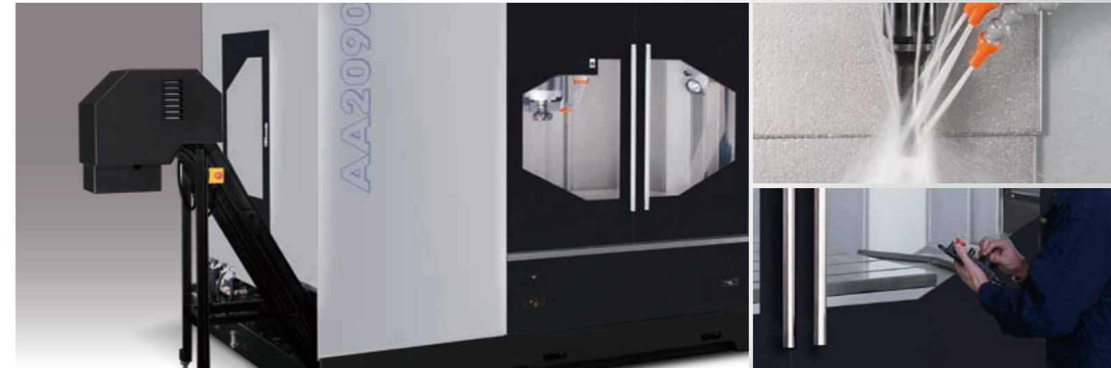
High performance chip discharge using Y direction screw type conveyors and X direction caterpillar type conveyor.
