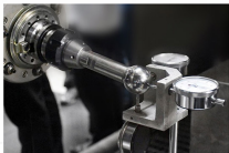
Detection of positioning accuracy 检测定位精度
