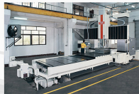
Five Face Double Column Machining Centre (Travel) 五面体龙门加工中心 (行程) : 6250mm x 2900mm x 1400mm
