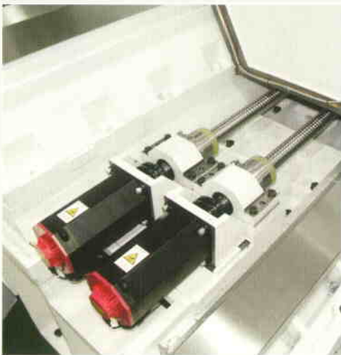
Patented Twin Ballscrew and Dual Feedback Technology (PAT. 8-355814)
