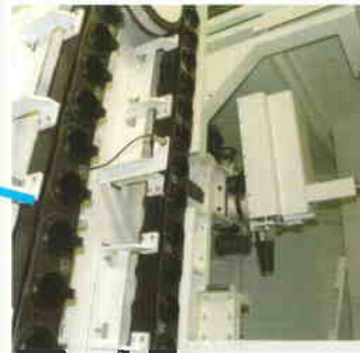
Sub arm feeds tool to swing pot.
