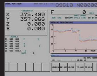
**Intelligent Advanced Control System.** Controls the effects of heat displacement in order to ensure continuous accuracy in machining. Minimizes head displacement to less than  $\pm 5$  microns. 6 sensors positioned on the machine measure and monitor temperature of machine and compensation guarantees positioning accuracy of  $\pm 0.002\text{mm}$  ( $\pm 0.000079''$ ) / Full stroke. Kitamura patented system since 1998.
