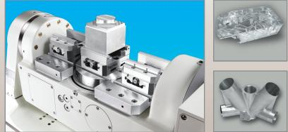
The integrated trunnion table offers the rigidity, accuracy and stability needed to productively machine complex part geometries. For those accustomed to 3-axis machining, the built-in table design of the tilting trunnion allows for high tech, high precision parts to be machined simpler and easier with less handling.
