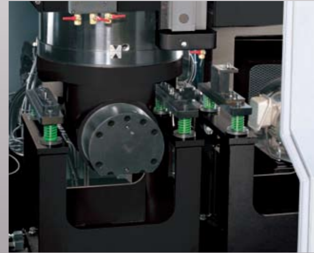
Horizontal Spindle exchange mechanism
