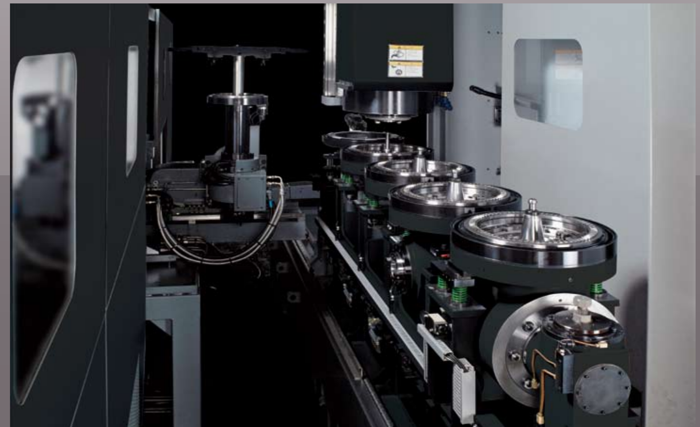
Automatic tool and head Storage system
