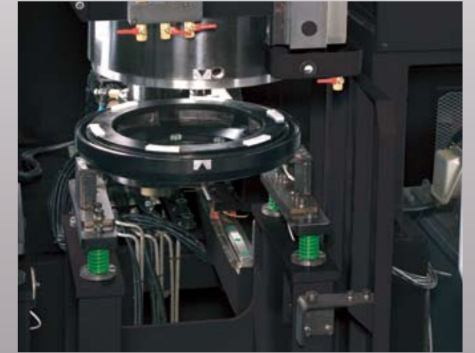
Vertical Spindle exchange mechanism
