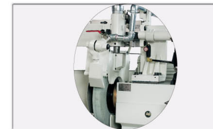
15. Wheel forming device (Manual type, without auto compensation)
