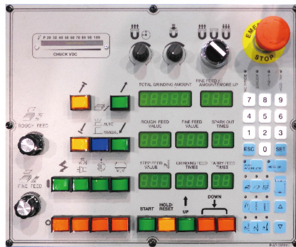
AUTOMATIC DOWNFEED AD5 (NC) CONTROL PANEL (optional)
