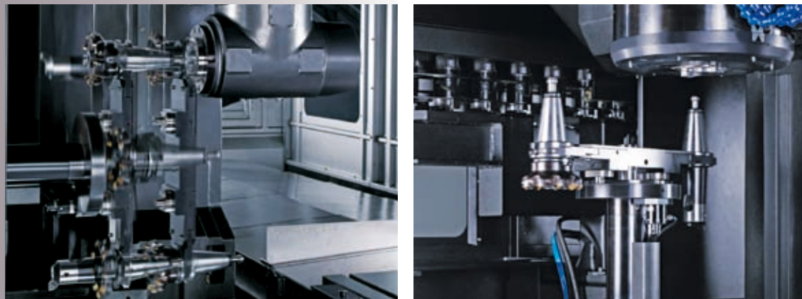
• Automatic tool exchange in horizontal. (chip to chip 50 sec.)
