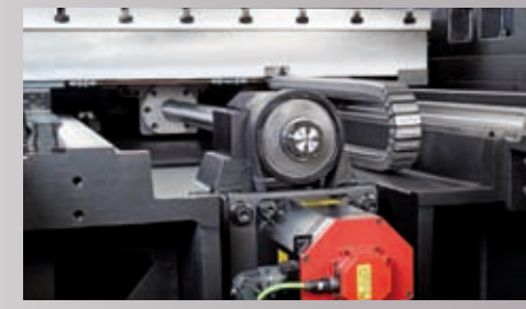
Torque limit mechanism in three axes.
