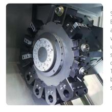
SL 2000M is equipped with standard 12-station BMT55 turret capable of accepting rotary tools at any station, providing flexible machining thru various machining operations in just one setup. Each BMT holder is securely tightened by 4 screws, allowing the turret to perform heavyduty cutting, milling and drilling operations. Turret indexing is non-stop,
