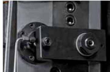
The W axis has been equipped with two sets/each sides of Hydraulic Clamping Cylinders for blocking the W axis wherever it located within full travel.
