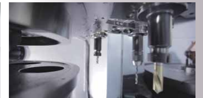
● Automatic tool exchange for vertical tools.
