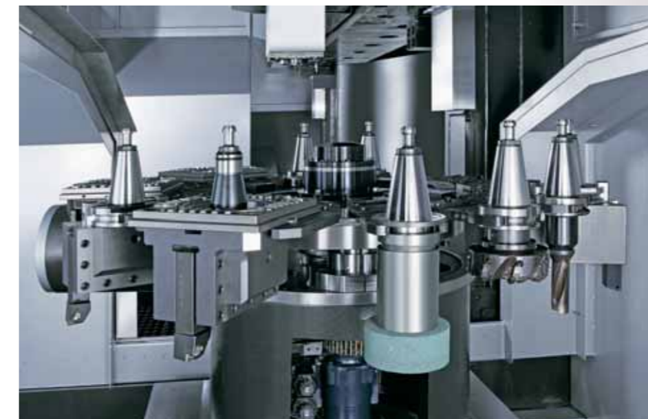
● 16 pockets tool magazine(STD) ; Two sets of curvic coupling attachment and 12 tools.
