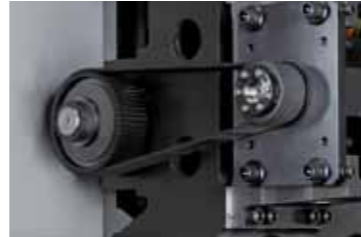
The X, Z and W axes with twin driver have equipped with the torque limit mechanism which protect the servo motors.
