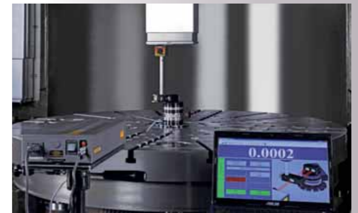
Cs axis rotation indexing positioning accuracy measurement.
