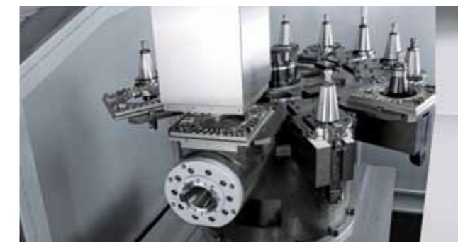
● Automatic exchange for multi-head attachment.
